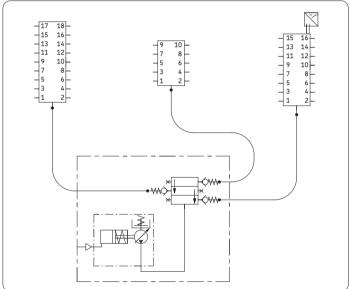
The control units described in this leaflet are used for time- or pulse-dependent control of central lubrication systems with progressive feeders.
