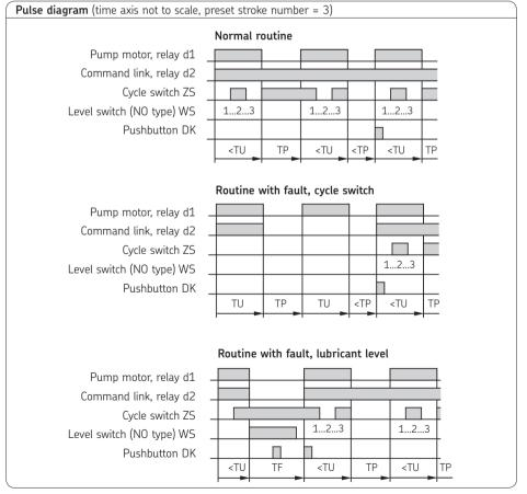
TU = monitoring time TN = pump delay time TP = interval time
