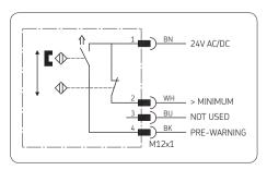
Illustration of contacts in wiring diagrams: reservoir filled to max. level.
