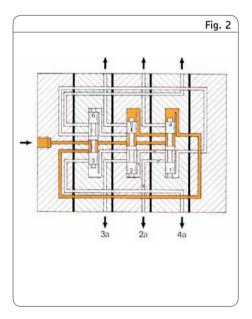
Piston end 5 has been actuated and piston end 2 delivers via outlet 2a. Next, piston end 6 will be actuated – and so on.
