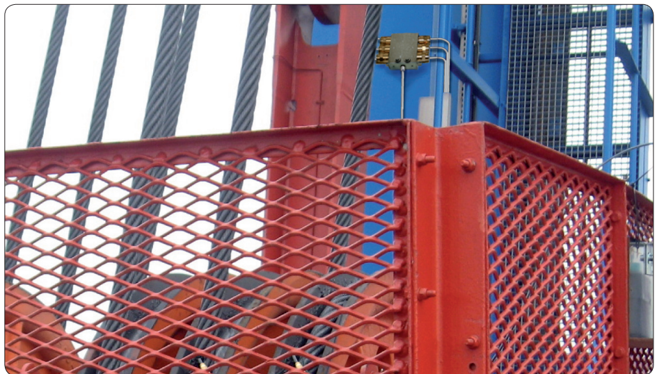
VPBM feeder, measures the lubricant according to the required lubricant quantity
