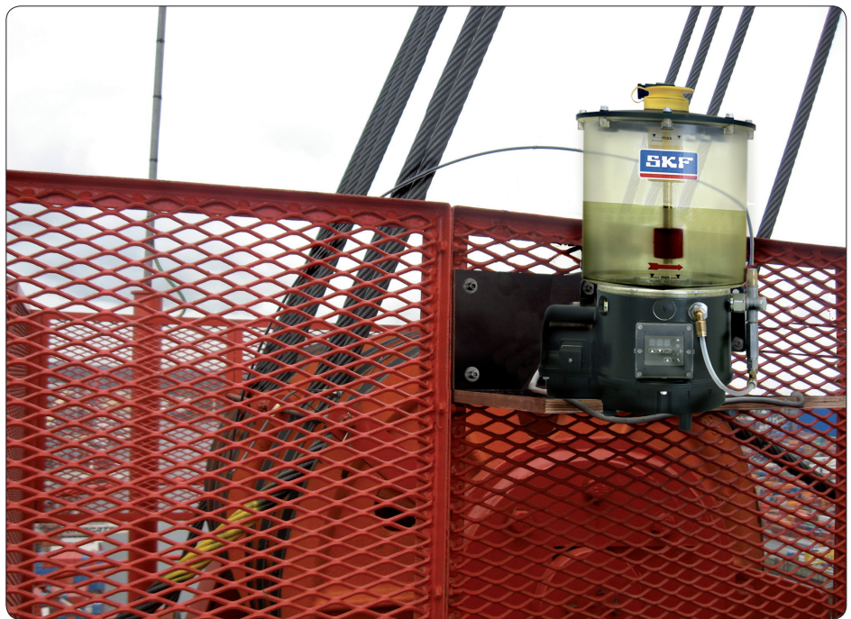
KFGS pump unit for oil, delivers the lubricant to the progressive feeders
