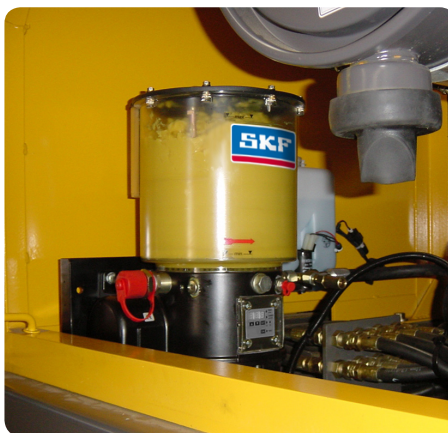
KFGS piston pump with 6 kg grease reservoir
