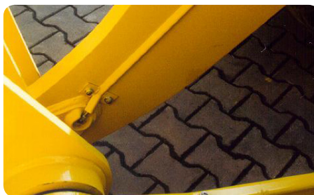
Especially exposed lubrication lines, e.g. in the shovel area, are protected by sectional steel.
